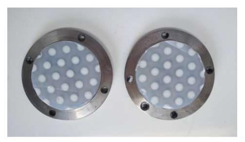
Pictures of sample of HI 3 sliding material after the execution of the test in combination with stainless steel plate at 60MPa contact pressure.
